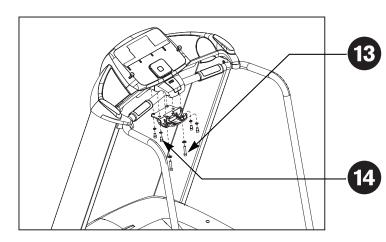
Replace the lower handrail clamp and secure the handrails to the clamp using two socket head screws (E) and two washers (F).
